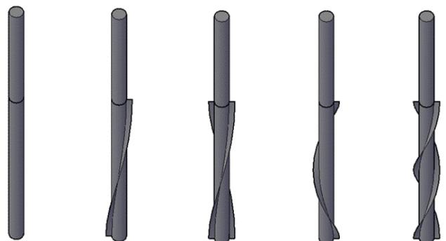
**Gambar 2.** Detail Model Pondasi Tiang Sirip
