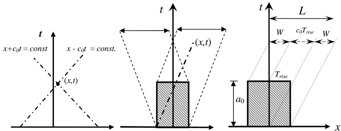
**Fig. 1** Illustration of  $(x, t)$  plane of generation region and interpreting wavelength.
