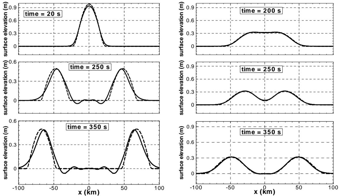
**Fig. 3** Generated tsunami profiles for Case 1. Left panel shows results of bottom motions with  $T_{rise} = 20$  s and the right panel shows results of bottom motion with  $T_{rise} = 200$  s simulated by: NLSW model (dash lines) and WNB model (solid lines).
