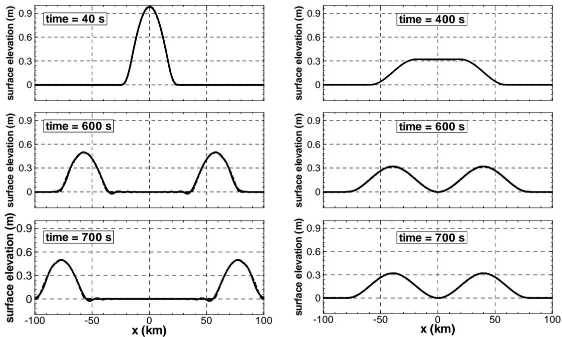
**Fig. 4** Generated tsunami profiles for Case 2. Left panel shows results of bottom motions with  $T_{rise} = 40$  s and the right panel shows results of bottom motion with  $T_{rise} = 400$  s simulated by: NLSW model (dash lines) and WNB model (solid lines).
