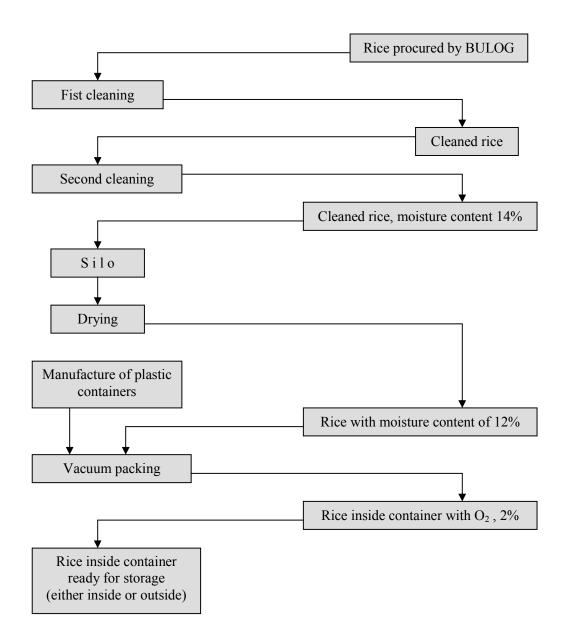
Figure 1. Schematic diagram of the vacuum process used for the modified atmosphere storage of milled rice
