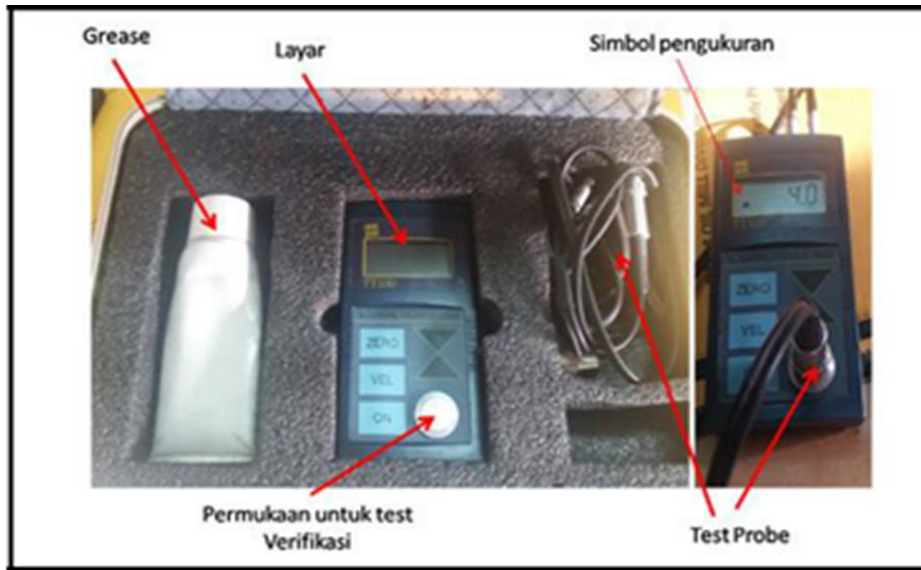
Gambar 4. Smart Sensor Ultrasonic Thickness Gauge TT 130
