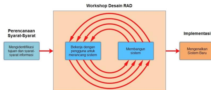
Gambar 2. Tahapan RAD (Rapid Application Development)
