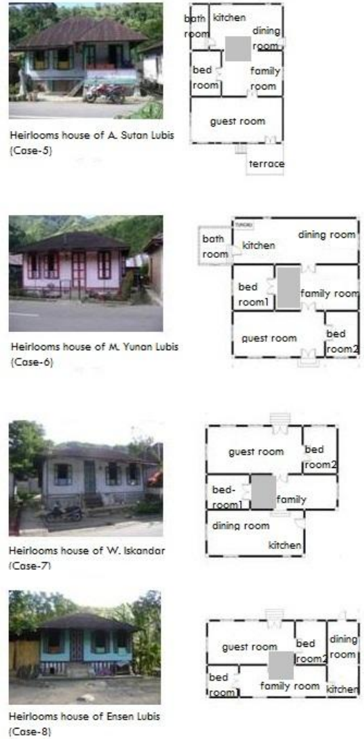
Figure 4. The position of pantar tonga (middle room as family room) in other four heirloom houses (C5-C8)
