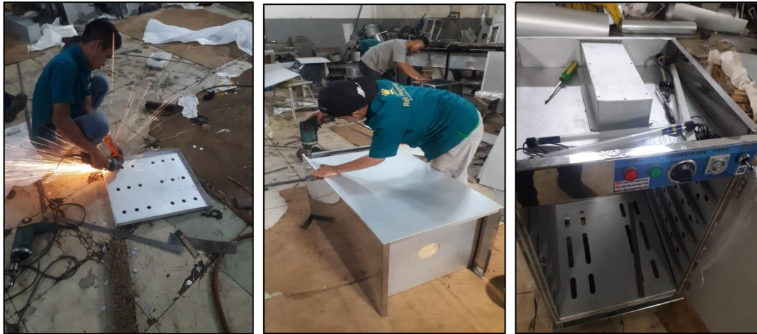
Gambar 6. Perakitan alat cabinete dryer sago sugar
