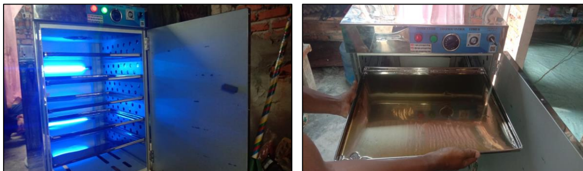
Gambar 7. Uji coba alat cabinete dryer sago sugar
