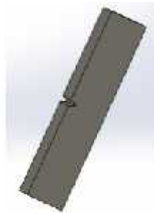
Gambar 3.2. Gambar 3D Detail spesimen plastik Uji pukul Charpy
