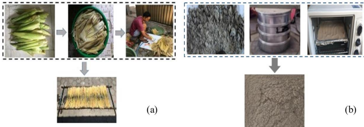
Figure 1. The extraction of corn husk fiber (a) and the treatment of pumice particles (b).
