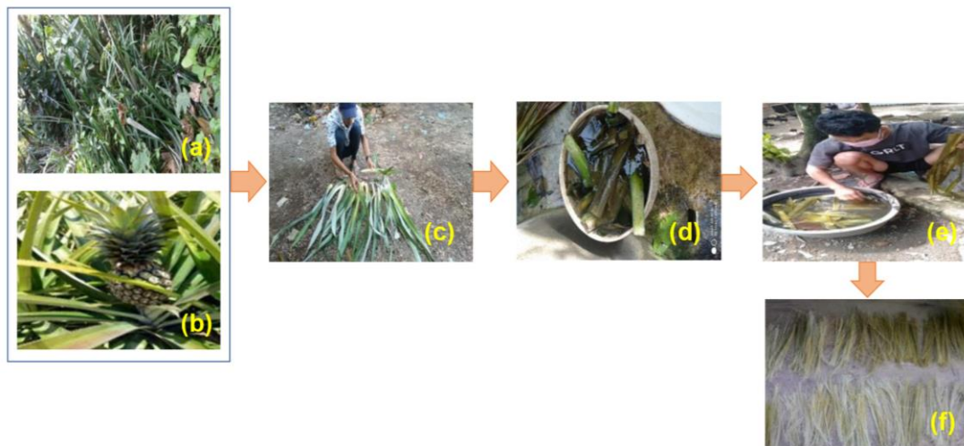
Figure 1. The extraction process of pineapple leaf fibers, a) and b) pineapple plant, c) pineapple leaf, d) soaking leaves in water, e) combing the leaves to pick up the fiber, and f) pineapple leaf fiber
