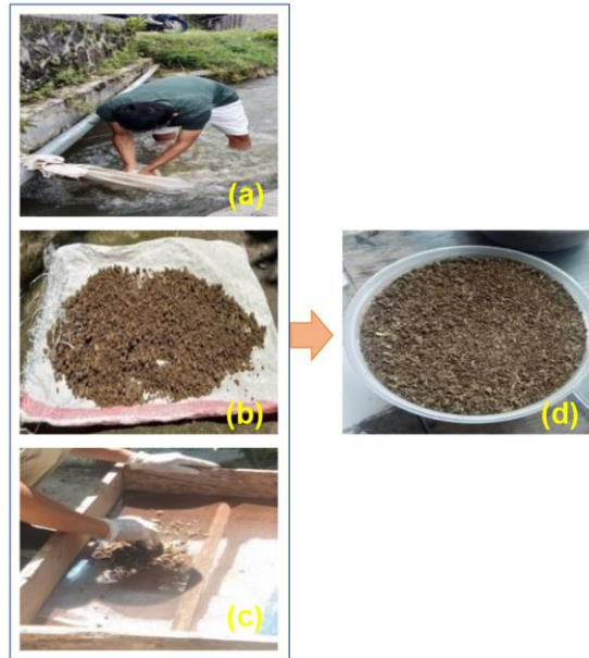
Figure 2. Extraction process of Horse dung particle, a) horse dung (HF), b) HF dried, c) sieving process, and d) HF particles.
