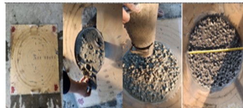
Gambar 2.3 Proses test slump flow beton umur 24 jam
