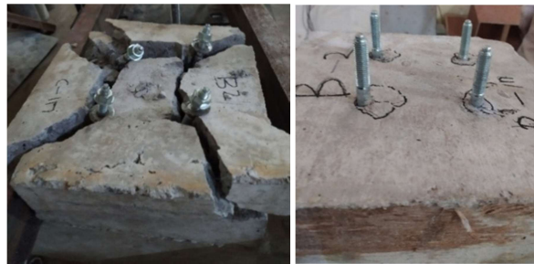
Gambar 6. Benda Uji Pasca Pengujian secara cast in place dan post installed
