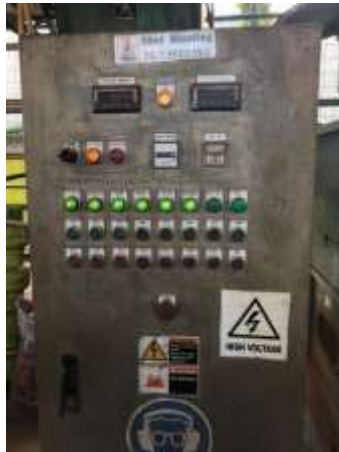
Gambar 7. Panel Kontrol Shotblasting Machine (Tochu) TG-7.5 FTJ
