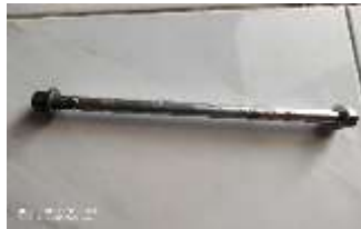
Gambar 2. Poros Roda Depan Vixion Advance 150cc 2015.
