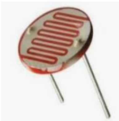
Gambar 2. LDR (Light Dependent Resistor)
