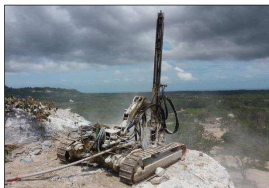
Gambar 4. CRD Furukawa alat bor PT Vitrama Properti
