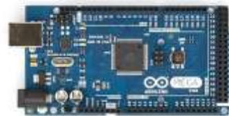
Gambar 2. Modul Arduino Mega 2560
