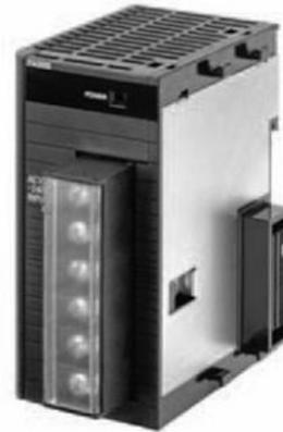
**Gambar 4.** Modul *power supply* CJ1W PA201
