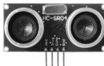
**Gambar 9.** Sensor ultrasonik HC-SR04 (Syam, 2013)
