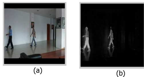
Gambar 5: Merubah frame RGB to Gray (a) Frame RGB (b) Frame Gray
