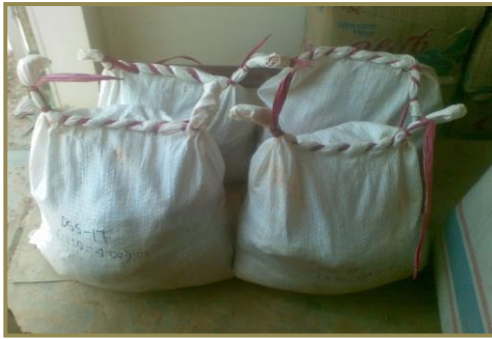
Gambar 5. Material disturbed sampling Sumber : Foto lapangan
