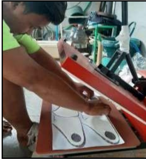
Figure 5 The Cutting Fabric into a Mask Shape with a Manual Pound Press Machine (Source : UMKM Cahaya Printing, 2020)
