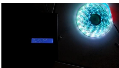
Gambar 7. Kondisi LED Strip ketika tombol Remote IR 2 ON
