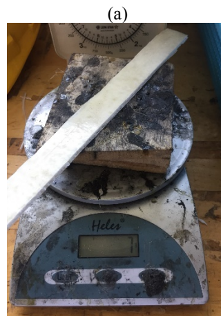
Gambar 9. (a) spesimen hasil hand lay-up (b) spesimen hasil vacuum bag
