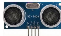
Gambar 2. Modul Sensor Ultrasonik (Sumber : Wicaksono, 2009)
