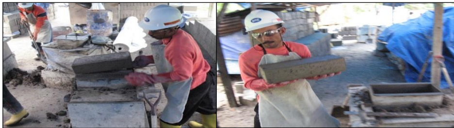
Fig. 5. Detachment Process from Mould
