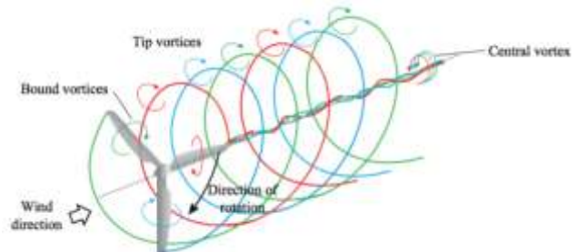
Figure 1. The formation of wind turbine vortex [13]
