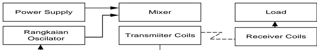
**Gambar 2.** Blok Diagram Sistem *Inductive Resonant Coupling*
