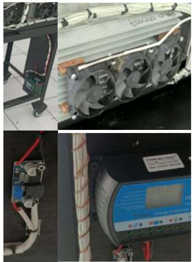
Gambar 11. Akumulator, step up tegangan, charger akumulator, dan kipas pendingin.
