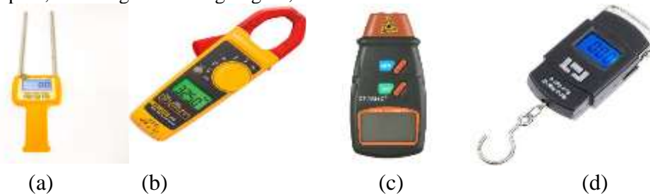
Gambar 21 a) Moisture Meter, b) Tang Ampere, c) Timbangan Gantung Digital, d) Tachometer
