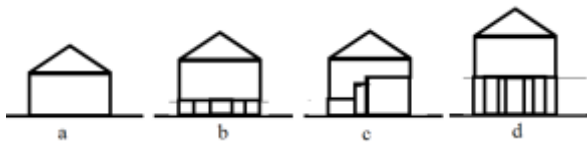
Fig. 3. Typology of Indonesian vernacular houses based on distance from the ground. From left to right: (a) house embedded to the ground, (b) house with low pit, (c) house with split level floors, (d) house with large pit, accessed by standing human.
