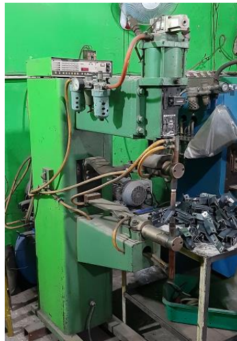
Figure 3. Machine Las Spot/Stationary Spot Welding
