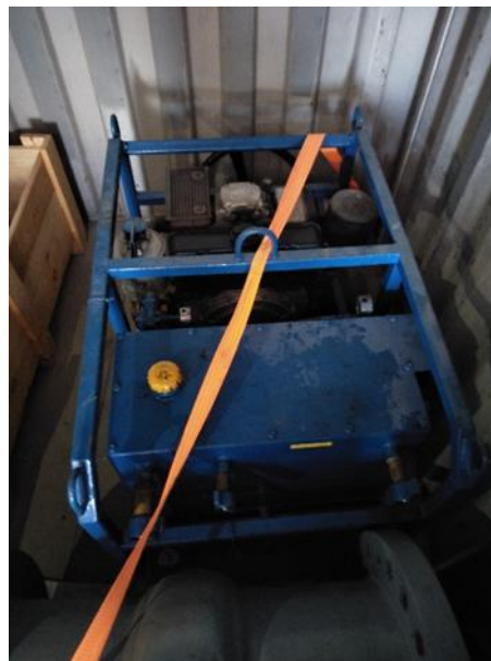
Gambar 5 Hydraulic Power pack
