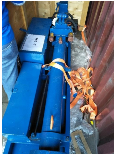
Gambar 2. Alat Hot tapping 760 TDW
