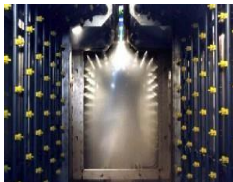
Gambar 2. Pre-treatment powder coating[2]
