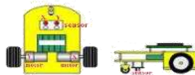
Gambar 6 Contoh Rancangan Mekanik Line Follower Robot [11]
