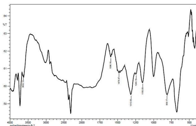
Figure 4. 5-minute polyaniline FTIR spectrum
