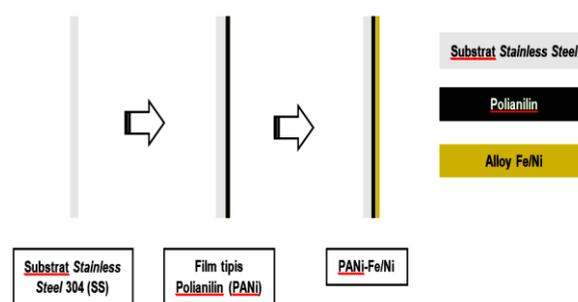
**Figure 1.** Fe/Ni Alloy Electrodeposition Scheme
