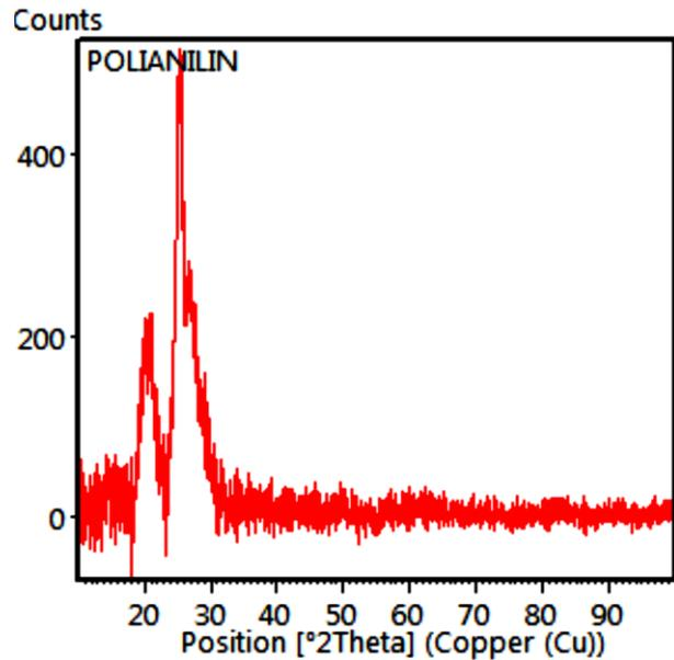
Figure 7. Polyaniline X-ray Diffraction Pattern
