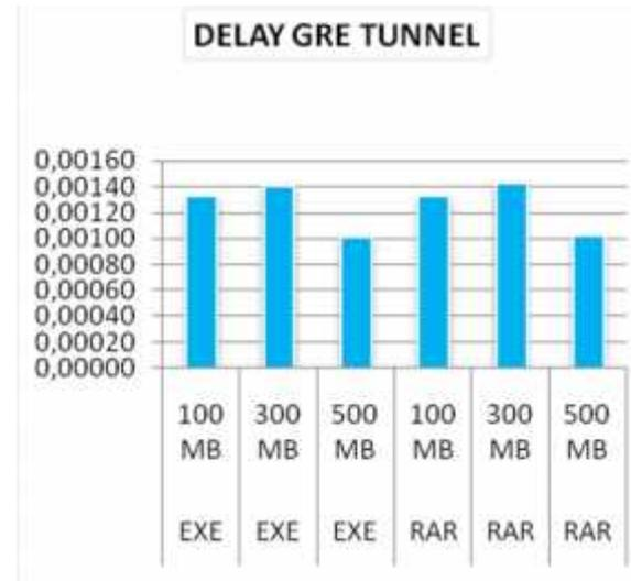
Gambar 5. Grafik Delay GRE Tunnel
