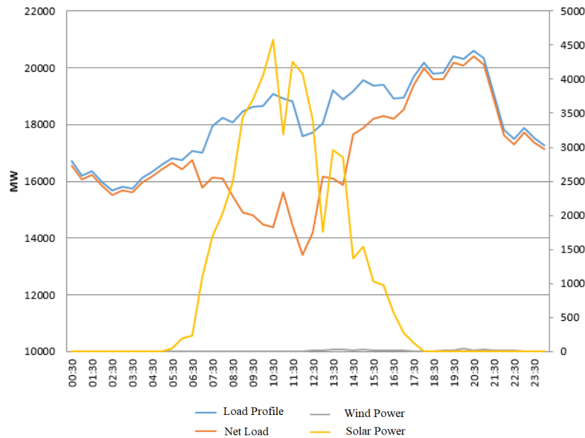
FIGURE 6. IRES Generation Penetration Projection \pm 20\% from Peak Load
