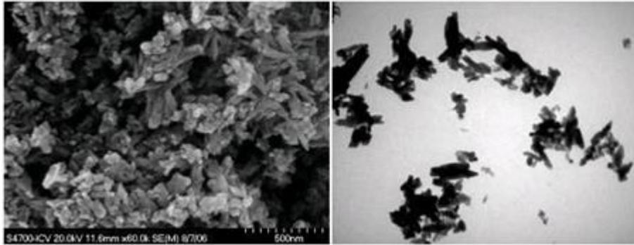
Figure 2. SEM (Left) and TEM (Right) *Micrographs*. Nanocrystal Morphology Characteristics in Hydroxyapatite Nanoparticles. Nanoparticle's size 80x20(SEM, *scale bar*=500nm; TEM, 12000x)<sup>34</sup>
