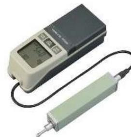
**Gambar 4.** Surface Roughness Tester Mitutoyo SJ 201P
