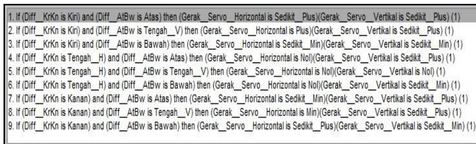
Gambar 12 *Rule base system dual axis solar tracking*
