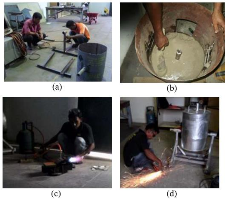
Fig 2. The furnace fabrication process: (a) assembling the frame and body; (b) using the refractory cement; (c) testing the burner; (d) the body and the frame of the furnace assembled.
