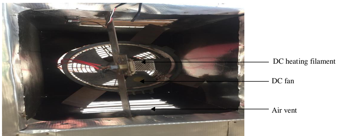
Figure 2: Hot-air supplement section of the dryer
