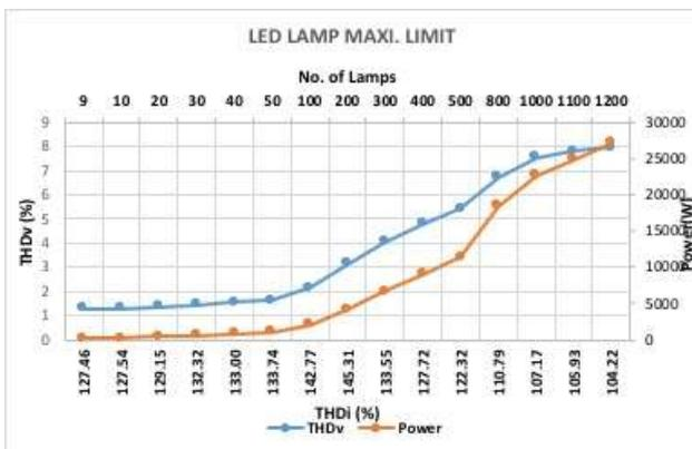
Fig. 13 Maximum possible power loading limit of LED lamps
