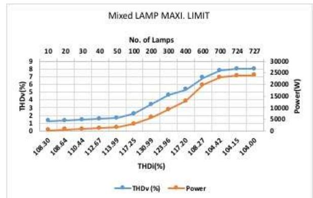
Fig. 11 Maximum possible loading limit of CFL lamps
