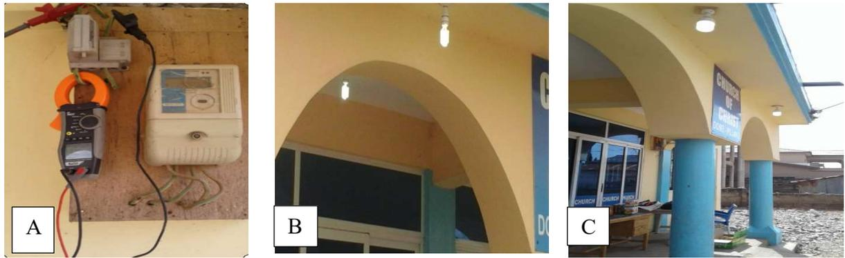
Fig. 1 Field measurement at facility PCC: A – power quality analyzer HT 9022 captures data and sends by Bluetooth to laptop, B– 23W Focus CFL lamps in installation, C – 20W Ant Electrical LED lamps in installation
