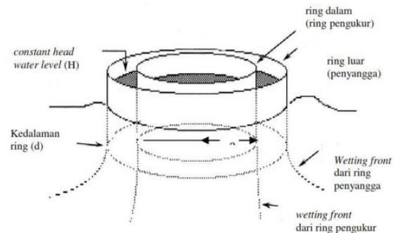
**Gambar 1.** Double Ring Infiltrometer
