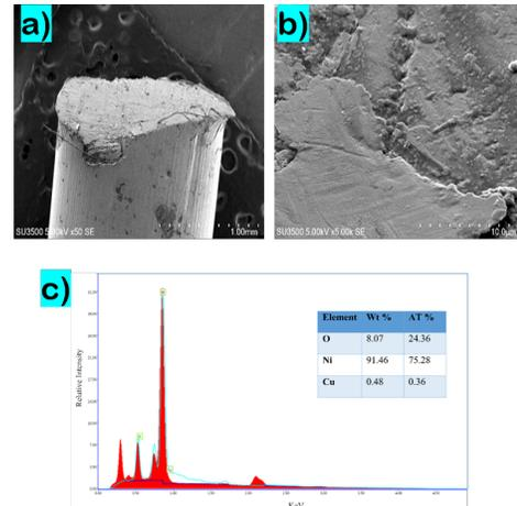
**Figure 3.** Morphology Scanning Electron Magnetic (SEM) of Material Ni/EC Surface with Magnification 5 Times (a), 5000 Times (b) and Result of Energy Dispersive X-Ray (EDX) from SEM Data Surface Electrode Ni/EC (c)
