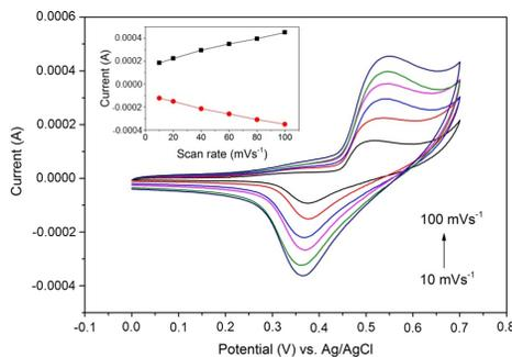
**Figure 8.** Cyclic Voltammogram of Various Scan Rate (10-100  $\text{mVs}^{-1}$ ) in 0.001 M Glucose
