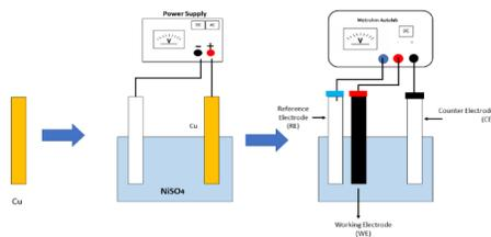
**Figure 1.** Schematic of Nickel Electroplating on Copper
