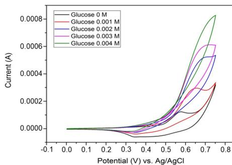
**Figure 5.** CVs of Ni/EC Electrodes in NaOH 0.1 M at Different Glucose Concentrations Scan Rate of 100 mVs<sup>-1</sup>
