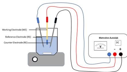
**Figure 2.** Electrochemical Cell
