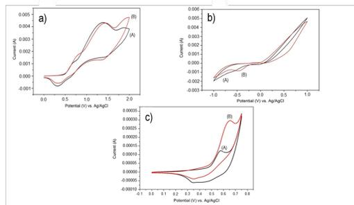
**Figure 4.** CVs of Ni/EC Electrode in Absence (A) and Presence (B) of Glucose 0.001 M in (a) KOH 0.1 M solution, (b) KNO<sub>3</sub> 0.1 M solution and (c) NaOH 0.1 M Solution. Scan Rate 100 mVs<sup>-1</sup>
