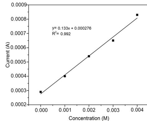
**Figure 7.** The Corresponding Calibration Curve of Ni/EC Electrode
