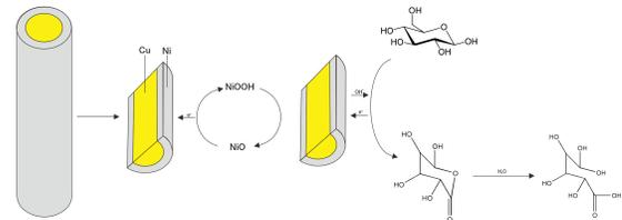
**Figure 6.** Reaction Possible of Glucose in Surface Ni/EC Electrode
