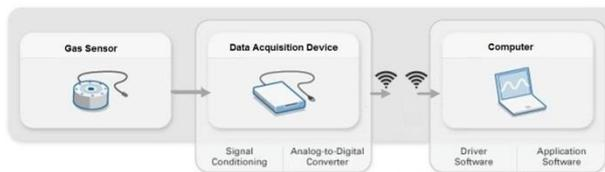
Figure 1 The Block Diagram of Alcohol Classification
