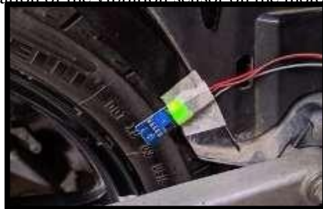
Figure 3. Installation of infrared sensors on motorcycle wheels
