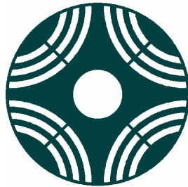
Figure 1. Modern Transverse Lamination Rotor for SynRM
