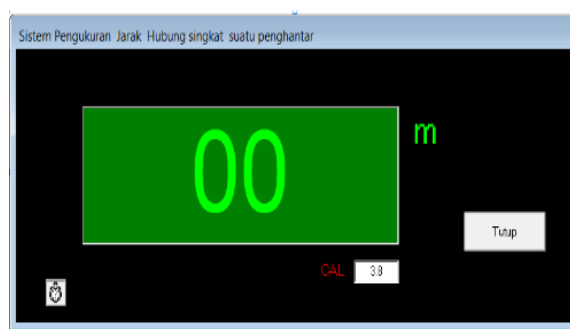
Figure 7. display of short circuit location measurement
